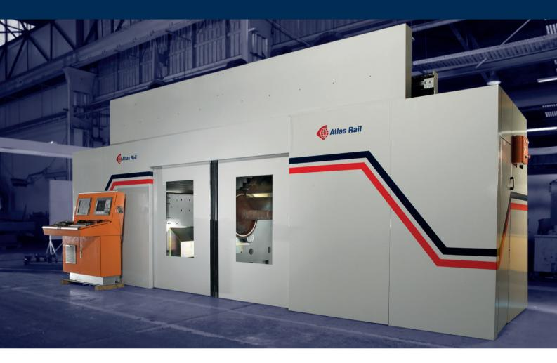
The Atlas Rail PS-2600 portal wheel lathe has been designed for re-turning operations for a wide variety of wheelset types and gauges. Designed in consultation with Australia's largest wheelset maintainers.
