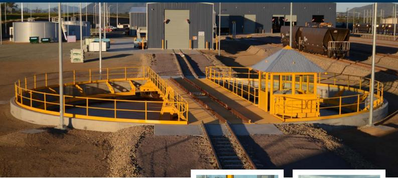
The Atlas Rail Locomotive Turntable is designed for 180 degree rotation of rolling stock up to 180T capacity. The turntable allows fast and efficient rotation of rolling stock without the need for extensive track work or occupying valuable surface area.
