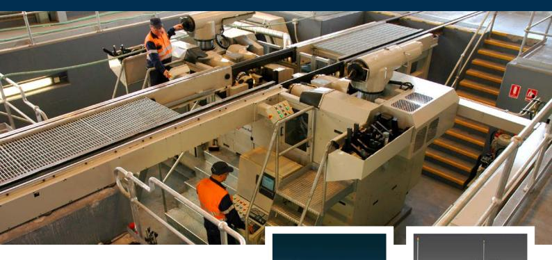
The Atlas Rail Underfloor Wheel Lathes (UFWL) are designed to re-profile wheelsets both on and off the vehicle for a wide range of rolling stock. It is a heavy constructed proven machine, designed for years of use and is in service with many rail operations around the world.
