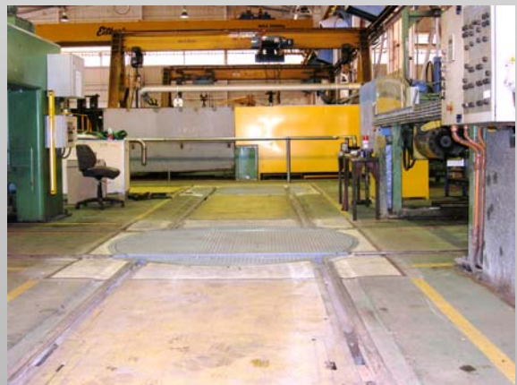
Two turntables feeding a Bearing Press and a Wheel Qualifying Machine
